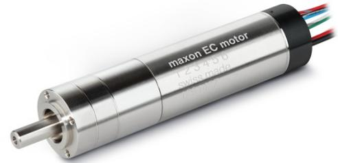
With maxon motor's winding technology, it is possible to offer various voltage versions. The stator has been designed without slots. Therefore, no cogging torque occurs resulting in excellent control properties and extraordinarily smooth running. Together with an optimally balanced rotor, low-noise and low-vibration operation is easily achieved.
