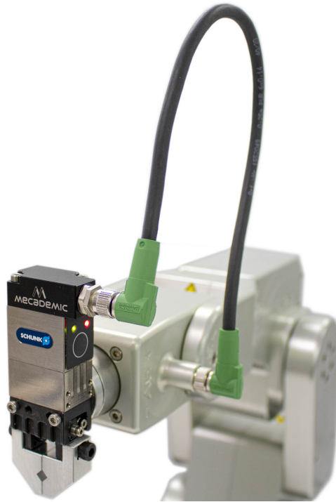
Figure 6: The MEGP 25E completely installed and homed
