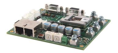
The **FD060-5-CM** is a servo drive and development board assembly for a FE060-5-CM FlexPro<sup>®</sup> series servo drive with IMPACT<sup>TM</sup> architecture. Connections to the controller, motor, power, and feedback are simplified through the standard connectors featured on the board. The **FD060-5-CM** is ideal for prototyping and can be used in production and industrial environments as well.
