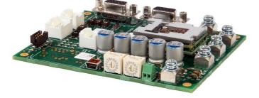
The **FD060-5-RM** is a serve drive and development board assembly for a FE060-5-RM FlexPro<sup>®</sup> series serve drive with IMPACT<sup>™</sup> architecture. Connections to the controller, motor, power, and feedback are simplified through the standard connectors featured on the board. The **FD060-5-RM** is ideal for prototyping and can be used in production and industrial environments as well.
