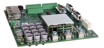
The **FD100-50-CM** is a serve drive and development board assembly for a FE100-50-CM FlexPro<sup>®</sup> series serve drive with IMPACT<sup>™</sup> architecture. Connections to the controller, motor, power, and feedback are simplified through the standard connectors featured on the board. The **FD100-50-CM** is ideal for prototyping and can be used in production and industrial environments as well.
