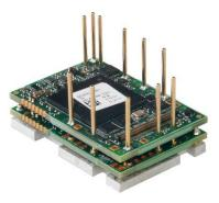
The **FE060-1-RM** is a FlexPro<sup>®</sup> series servo drive with IMPACT<sup>™</sup> architecture.
