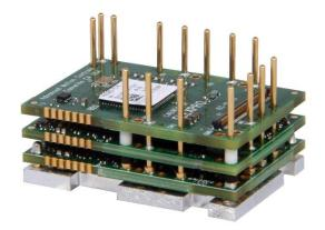
The **FE060-10-EM** is a FlexPro<sup>®</sup> series servo drive with IMPACT<sup>TM</sup> architecture.
