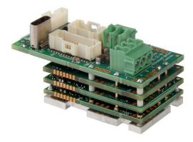
The **FM060-1-EM** is a single-axis servo drive and integration board assembly for a FE060-1-EM FlexPro<sup>®</sup> series servo drive with IMPACT<sup>™</sup> architecture. Connections to the controller, motor, power, and feedback are simplified through the standard connectors featured on the board.
