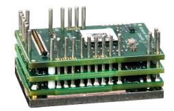
The **FXE060-5-EM** is a FlexPro<sup>®</sup> series Extended Environment servo drive with IMPACT<sup>TM</sup> architecture.
