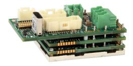
The **FXM060-10-CM** is an Extended Environment single-axis servo drive and integration board assembly for a FXE060-10-
