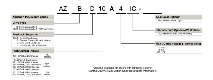
ADVANCED Motion Controls servo drives are available in many configurations. Note that not all possible part number combinations are offered as standard drives. All models listed in the selection tables of the website are readily available, standard product offerings.
