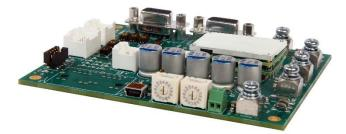
The **FD060-60C-CM** is a serve drive and development board assembly for a FE060-60C-CM FlexPro<sup>®</sup> series serve drive with IMPACT<sup>TM</sup> architecture. Connections to the controller, motor, power, and feedback are simplified through the standard connectors featured on the board. The **FD060-60C-CM** is ideal for prototyping and can be used in production and industrial environments as well.
