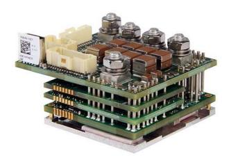
The **FM100-50-EM** is a single-axis servo drive and integration board assembly for a FE100-50-EM FlexPro® series servo drive with IMPACT<sup>TM</sup> architecture. Connections to the controller, motor, power, and feedback are simplified through the standard connectors featured on the board.
