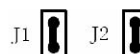
(d) J1 short circuit, J2 short circuit CW/CCW mode and effective at downward-falling edge
