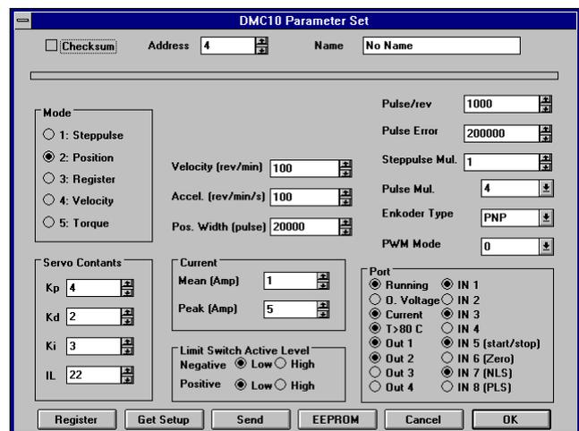
It is also possible to obtain a very quick overview of the set-up of your servo-controller. A window shows the most important set-up parameters. To adjust individual parameters, simply key-in the required value in the correct field and select SEND. The new value is then set up on the Controller. It couldn't be simpler.
