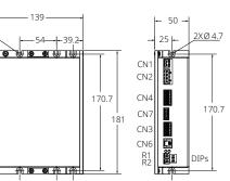
CN1: Power Supply CN2: Motor Connections CN3: Digital I/O CN4: Feedback Connections CN5A/5B: Modbus RTU Interface CN6: Service SCI Interface CN7: STO Inputs (mandatory
