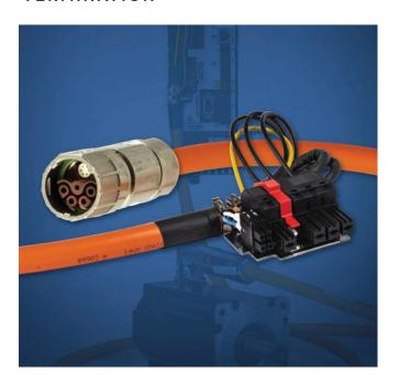
Any cable can fail prematurely, especially in a high-flex application, when it is not properly terminated. Termination-related loss of an electrical connection is one of the most common causes of system failures. Connector contacts should be rated for the wire size of the cable. If machine crimping is not available, use the proper hand tools to make reliable electrical and mechanical connections between the
