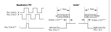
\*Output signals are differential. Inverse signals are not shown for clarity.
