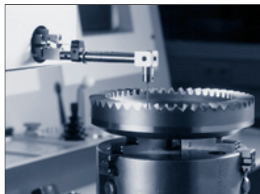
Computerized mapping of gear tooth profile
