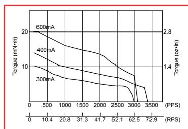
Coil Resistance: 16Ω Supply Voltage: 24V
