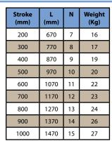
N = sets of holes on stage Available stroke 100mm-1800mm
