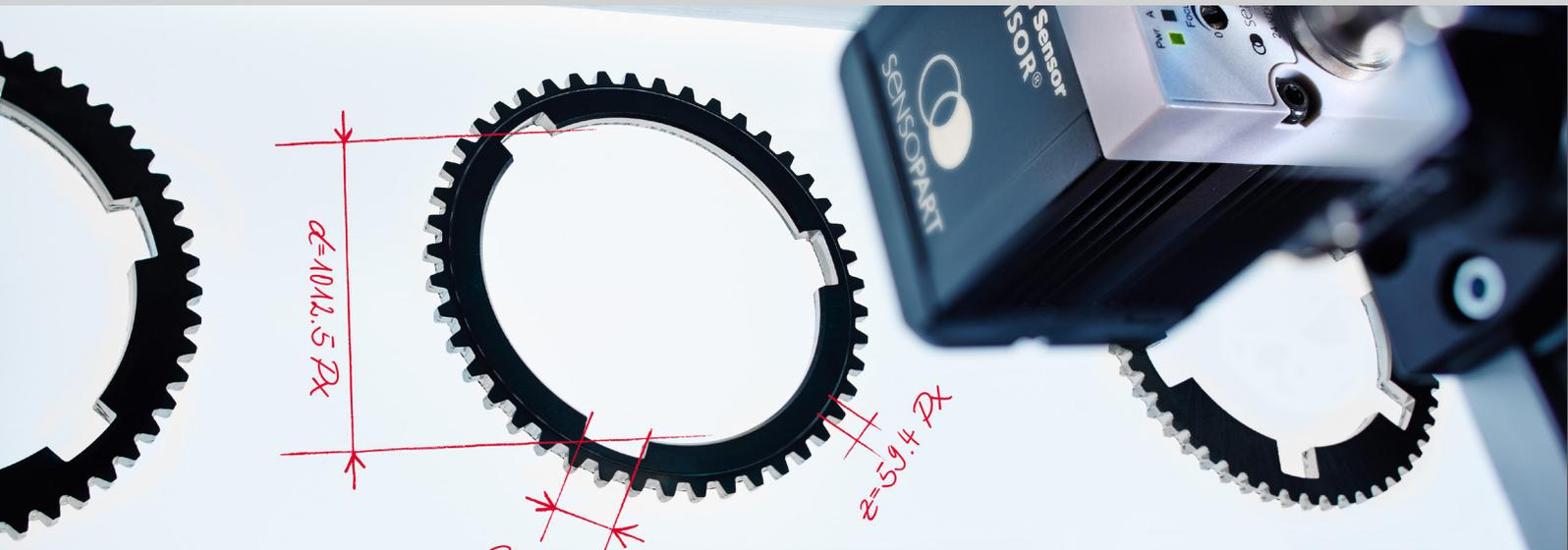
Component position and distance values are generally required in metric units, such as millimeters or inches, rather than in pixels. Thanks to the VISOR® calibration function, vision sensor coordinates can now effortlessly be converted into real-world engineering units: place the calibration plate into the sensor's field of view, a single mouse click in the configuration program – and it's done!
