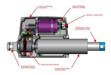
Electric actuator design has migrated from an approach that uses modular assemblies to one in which the key components are encapsulated in a "clamshell" that cradles them against shock and vibration for optimized environmental protection.
