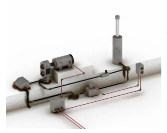
This single acting, uni-directional hydraulic cylinder system is one of the simplest hydraulic solutions available. It consists of eight parts that must be taken into consideration during the design process and installed by the OEM. For bidirectional operation, a more complex and costly bi-directional system would need to be installed.
