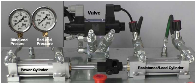
Illustrated above is how to measure pressure on both the blind-end and rod-end of the hydraulic cylinder.
