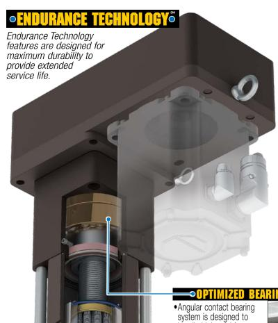
The RSX096P press actuator expands the extend force capability to 40,000 lbf (178 kN) making it well suited for applications such as pressing, riveting, clinching and many others. The RSX096P press model has all the features of the standard RSX on pages 4 & 5 plus oversized tie rods, a bearing system optimized for high force extend, and a high strength steel front flange.
