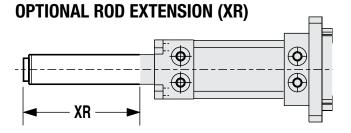
The thrust rod length can be extended by specifying the rod extension option. This does not increase the working stroke, only the length of the thrust rod.
