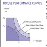
NOTE: Continuous torque specifications obtained with motor mounted to an 10"x10"x.25" aluminum plate at 25 C° ambient. Typical values are within  $\pm10\%$  of rating.
