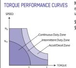
**NOTE:** Continuous torque specifications obtained with motor mounted to an 10"x10"x.25" aluminum plate at 25 C° ambient. Typical values are within  $\pm$ 10% of rating.
