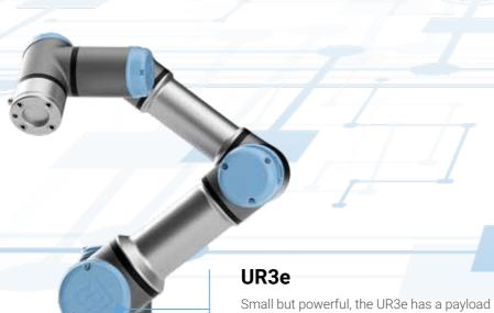
of 3 kg and reach radius of 500 mm. With 360-degree rotation on all wrist joints and infinite rotation on the end joint, this tabletop cobot handles high precision tasks and light assembly tasks with ease.
