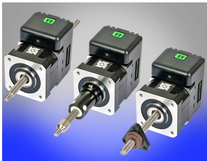
Fig. 9 Linear actuators with software programmable integrated drives, Size 17 non-captive, captive and external linear stepper motors with IDEA™ Drives
