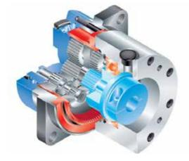
The HPF Harmonic Planetary® gear unit delivers hightorque and high-accuracy with a hollow shaft design. The gearhead incorporates continuous backlash compensation that ensures low backlash throughout the life of the gear. An extralarge cross roller bearing serves as the output flange and can directly support large loads with exceptionally high moment stiffness. The large coaxial hollow shaft allows cables, shafts, ball screws or lasers to pass directly through the axis of rotation.
