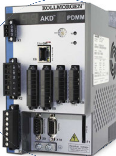
Control of motors with AKD ® PDMM programmable multi-axis master
